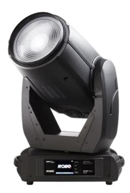
Mechanical features include a newly designed linear motorized zoom of 5.5° - 60° and a diffusion filter for extension of the zoom up to 75°. The fixture uses a internal Barndoor module for creating different shapes. The module consists of four individually controllable blades and is rotatable by plus or minus 90 degrees.
